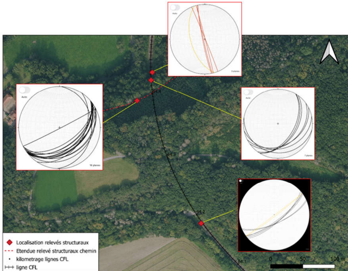
Figure 2. Variation of the strike and the dip of the stratification (black) all around the tunnel. The fault planes observed to the north of the tunnel are shown in red and yellow on the stereogram in the top center
