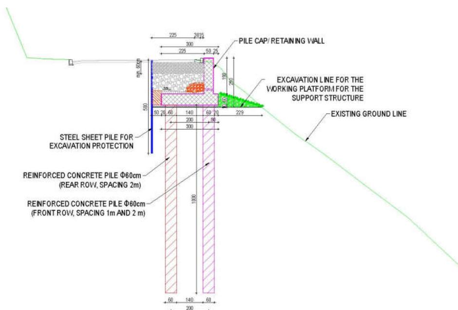
**Figure 20.** Cross-section with the planned landslide remediation solution
