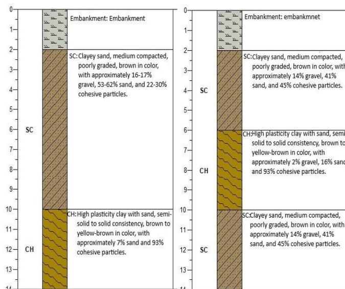
**Figure 19** Display of core samples from exploratory boreholes B1 (left) and B2 (right)
