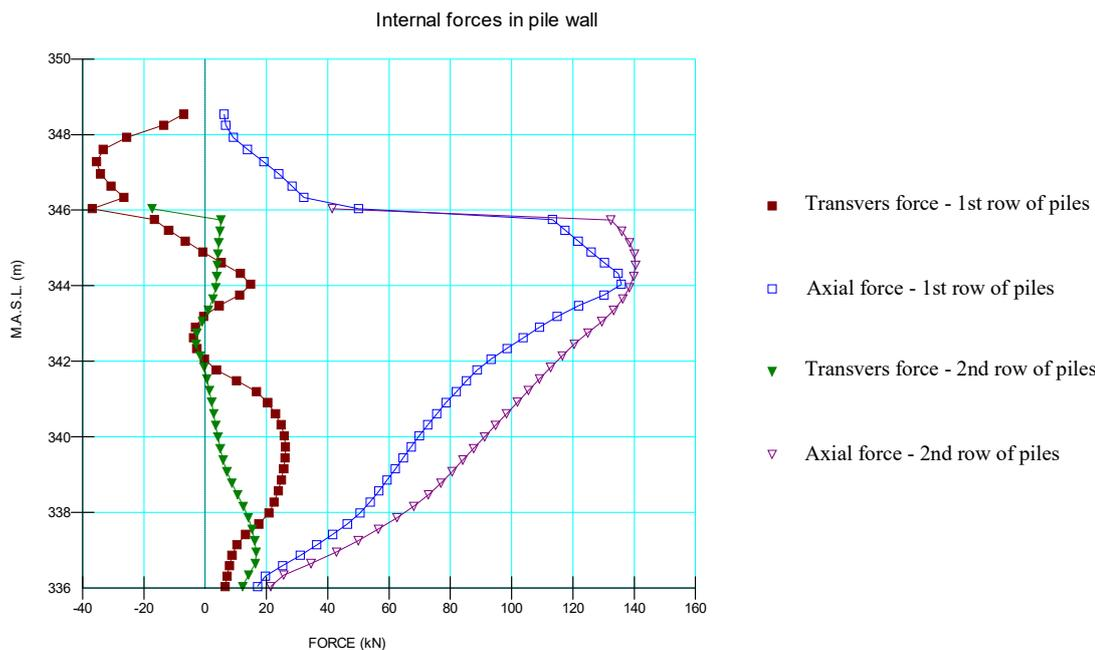
Figure 23 Transverse and axial internal forces of 1<sup>st</sup> and 2<sup>nd</sup> row of piles
