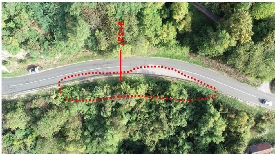
**Figure 16.** Area of instability and planned remediation, State Road DC206
